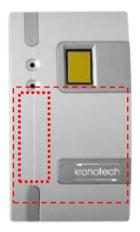
The window requests to use the card on the reader to store the fingerprints: the image on the left shows the reading area of the reader. Do not remove the card during the read/write operations.
